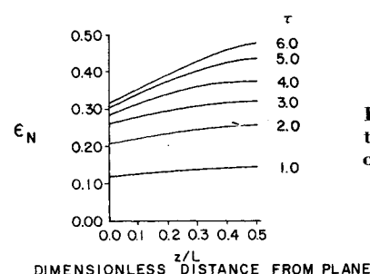
Fig. 10b Increase in normal emittance as a function of refractive index and optical thickness: \sigma = 0.95 .
